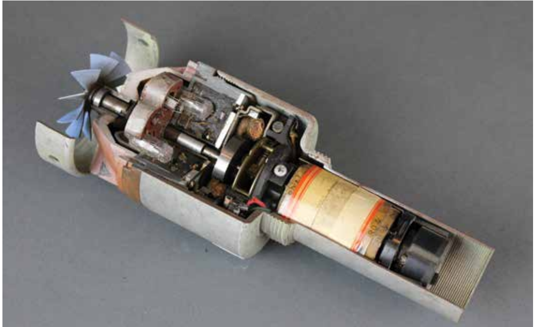
The proximity fuze caused a shell or bomb to explode when it got close to its target, rather than requiring an impact.
